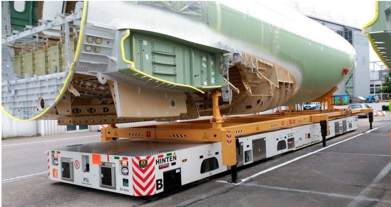
Figure 2: DTA Dolphin AGV transports aircraft fuselage at Acerinox in Spain. Courtesy: Bluebotics
