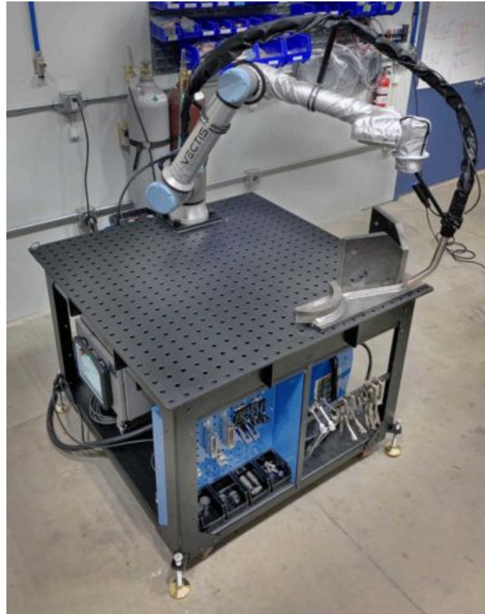
Figure 1: The Vectis Automation's ArcPilot is a through-the-arc seam tracking feature in the Vectis Automation Cobot Welding Tool (a system powered by cobots from Universal Robots) to help manage variations. Through-the-arc seam tracking enables path correction during live welding by monitoring and using welding arc's electrical characteristics to make cobot path adjustments in microseconds. The heavy-duty XL version of the Vectis Cobot Welding Tool can handle multi-pass welds and large wire diameters, common applications that can benefit from through-the-arc seam tracking. Courtesy: Vectis Automation
