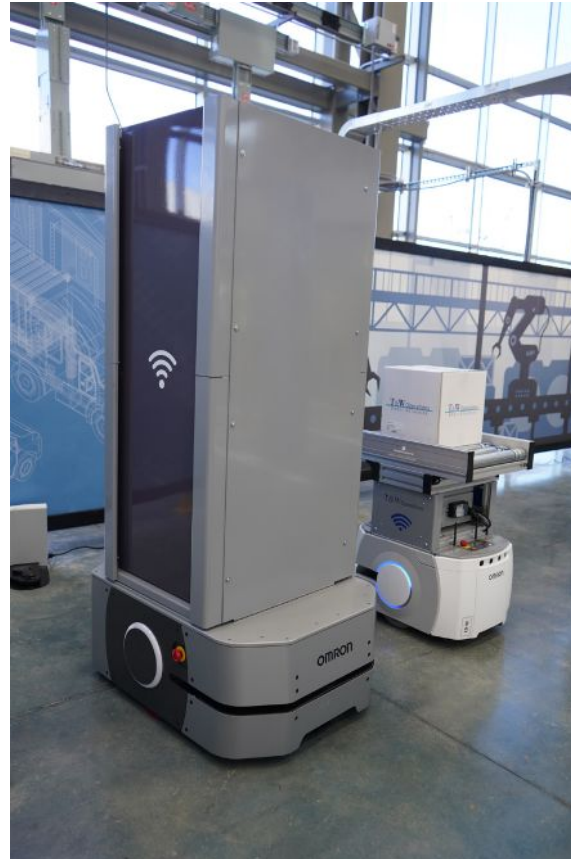
Figure 1: The T&W Expandable Robotic Tower Inventory System (TIS-ER) uses Omron Automation LD-250 mobile robot with a payload of up to 120 kg (265 lb) for a reach of 10 ft, and the Omron HD-1500 heavy-duty mobile robot with a payload of 1500 kg (3307 lb) for a reach of 30 ft. The mobile "tower" travels autonomously through warehouse aisles, collecting RFID tag data and communicating to the warehouse management system. Courtesy: Omron Automation
