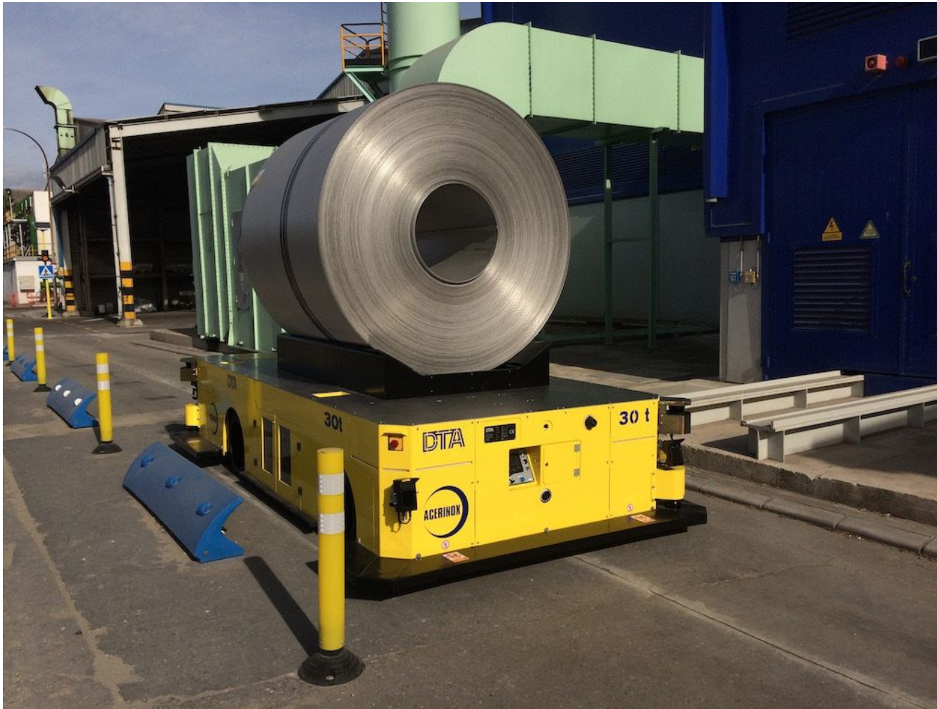
Figure 1: AGV transports steel coils at Acerinox in Spain. Courtesy: Bluebotics
