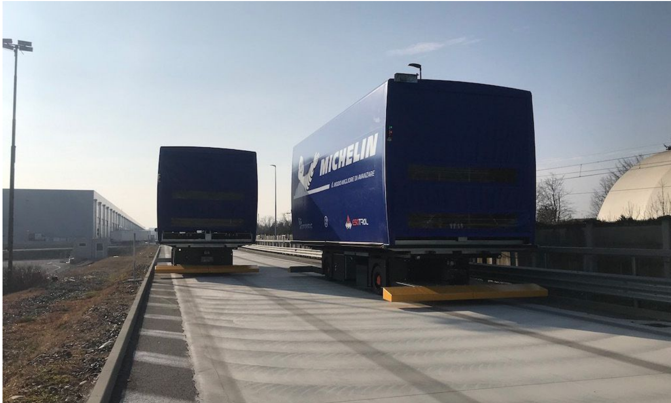
Figure 3: Esatroll AGVs move tires between buildings at Michelin's plant in Cuneo, Italy. Courtesy: Bluebotics
