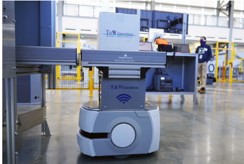
Figure 2: T&W's TIS-ER is designed to retrieve the container via the automated conveyor and proceeds to the RFID portal where the contents are again verified without human interaction. Courtesy: Omron Automation
