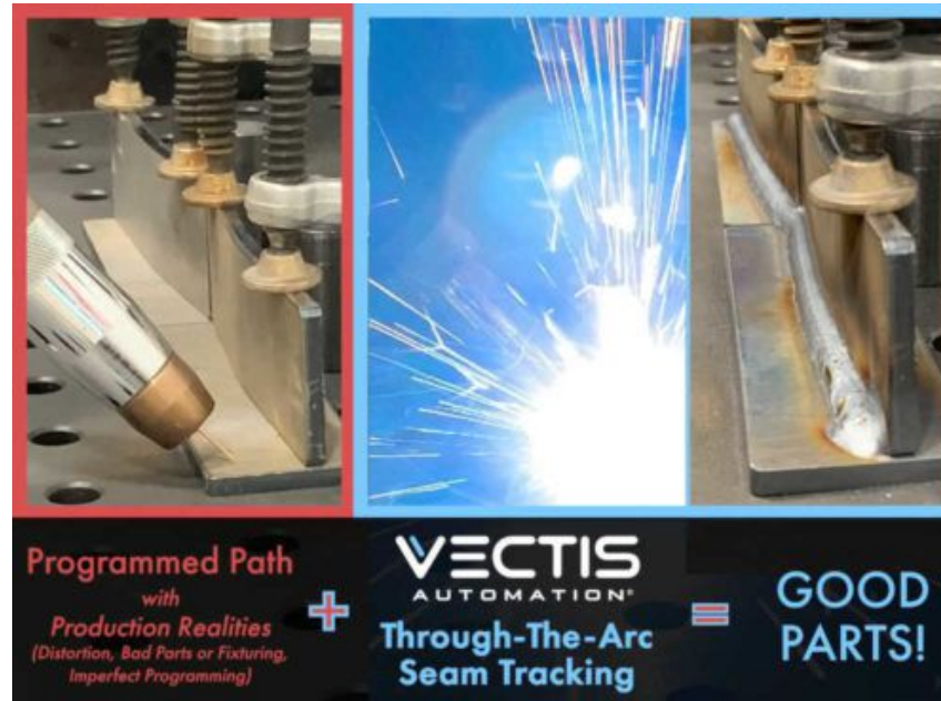
Figure 3: Vectis' ArcPilot through-the-arc seam tracking "steers" the cobot (left) along a symmetrical fillet joint, even with variances in the part relative to original programming, creating a high-quality, automated weld (right).
