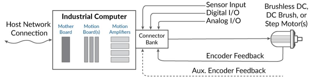
Figure 2A: Centralized motion controller architectures
