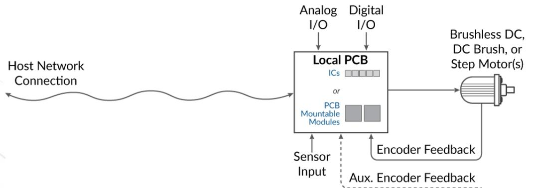
Figure 2B: Embedded motion controller architectures
