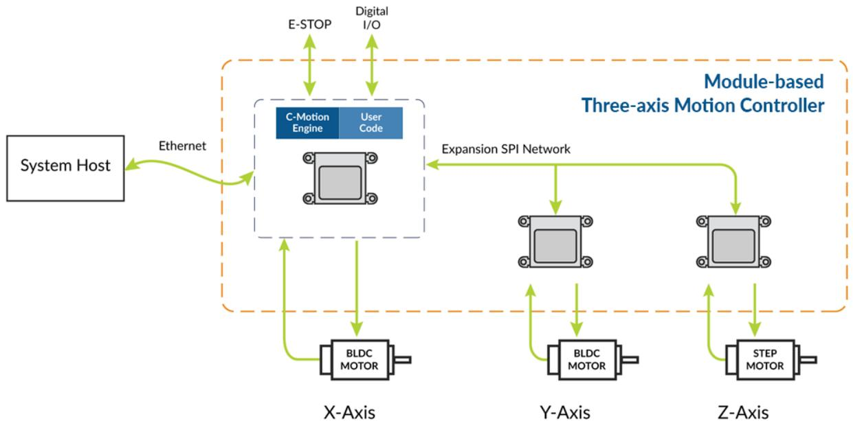
Figure 8: Control architecture for three-axis module-based controller PCB
