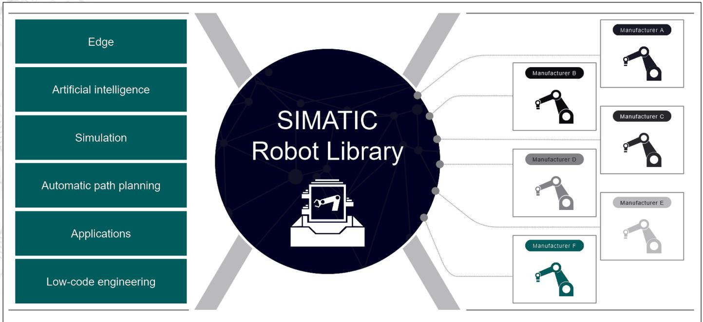
**Figure 4: The Siemens SIMATIC Robot Library empowers automation programmers to control robots within a single PLC using identical programming blocks regardless of robot manufacturer.**
