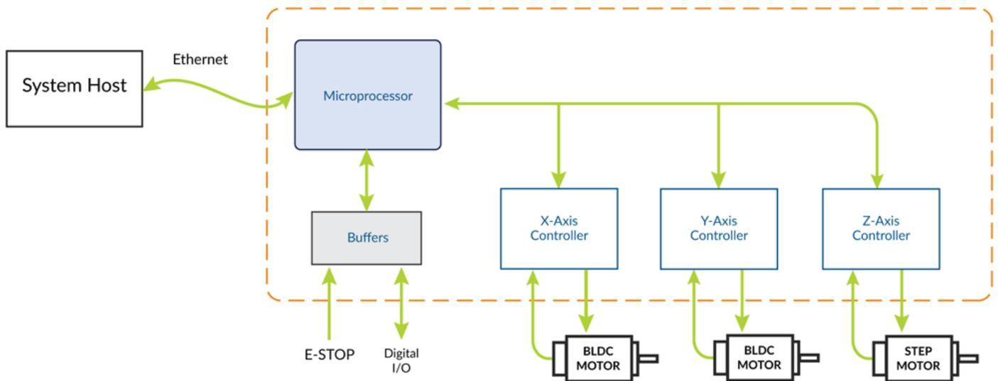
**Figure 3: Overall architecture of three-axis controller**
