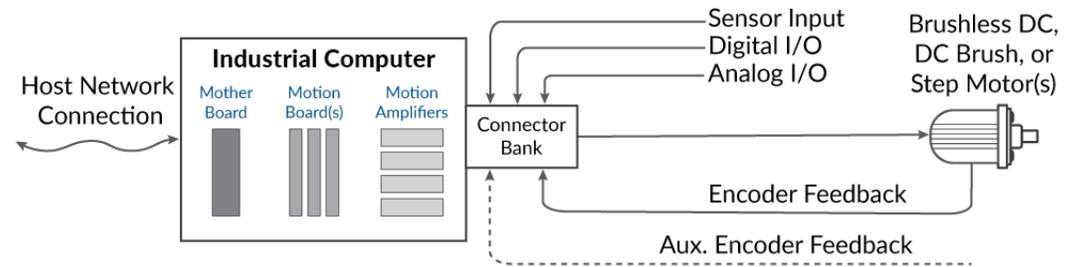
Figure 2A: Centralized motion controller architectures
