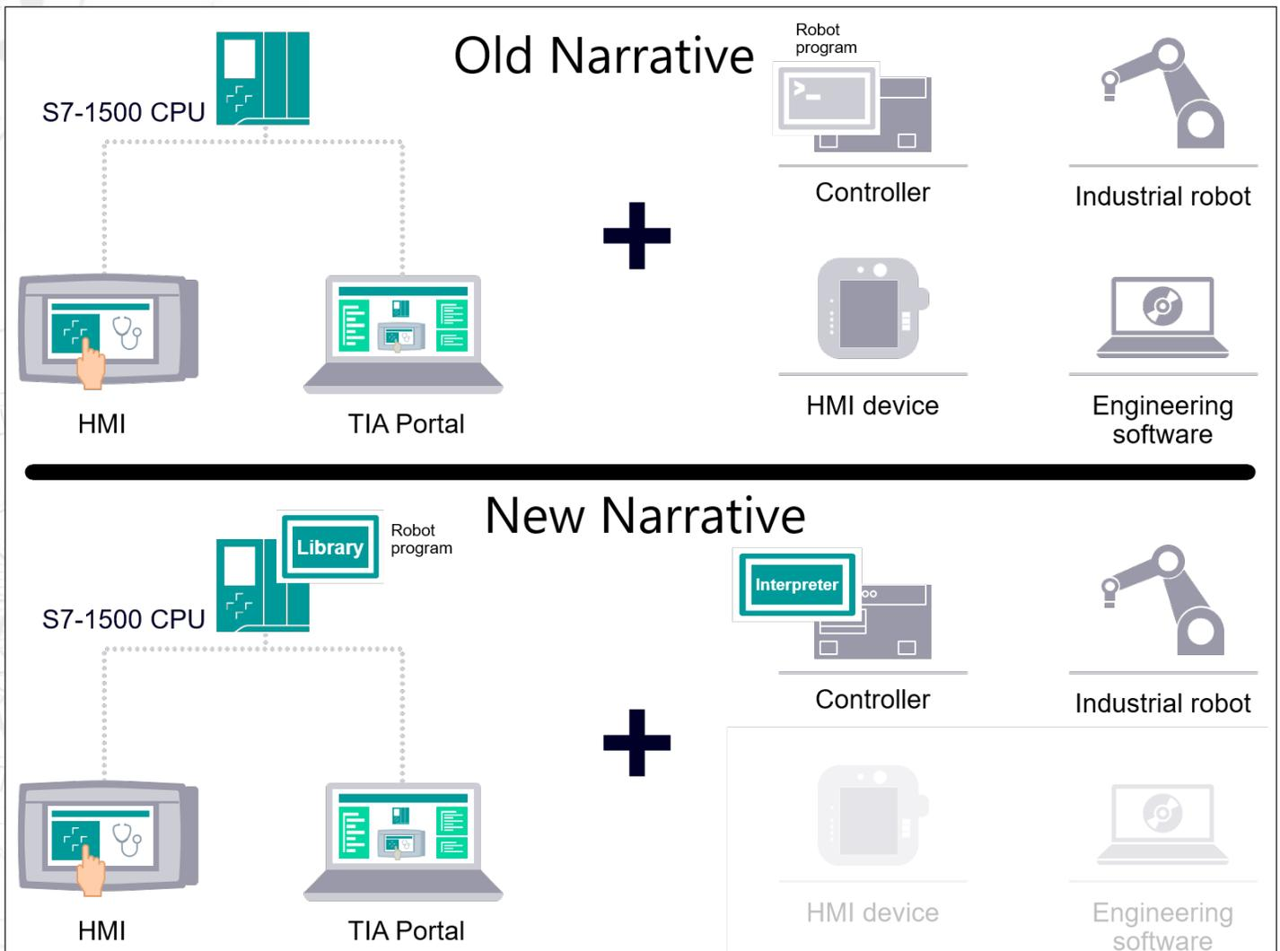
Figure 2: Siemens SIMATIC Robot Integrator software embeds robot control within a standardized PLC library, universal among multiple manufacturers' robots.
