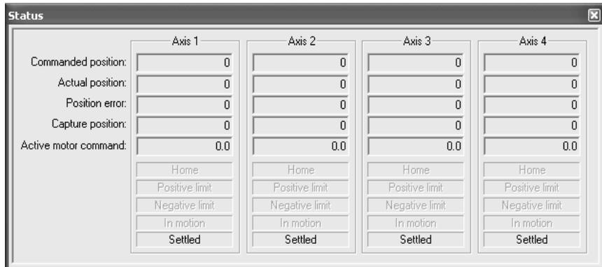
The Status window allows you to continuously monitor the values of selected motion processor registers. Status tracks the values of up to four axes in tabular form and displays the following data for each axis:
