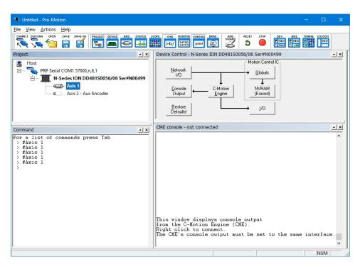
At the center of the screen you will see the **Device Control** window. This convenient graphical representation of the CME device allows you to manage card-level functions. The **Console** window is to the bottom. This will show messages output from the C-Motion Engine.
