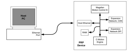
Figure 2-1: Host PC Connected to PRP Device via Ethernet TCP
