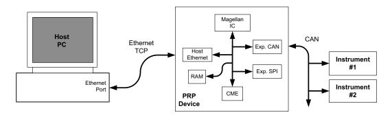
Figure 2-2: Host PC Connected to PRP Device connected to Instruments via CAN Network
