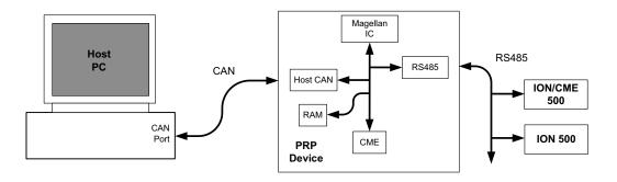
Figure 2-3: Host PC Connected to PRP Device connected to ION/CME and ION 500 via RS485 Network
