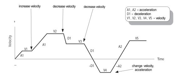
Figure 4-8: Velocity-Contouring Profile
