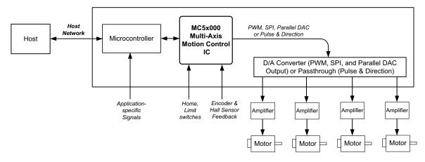
Figure 1-5: Magellan using Off-board Amplifiers
