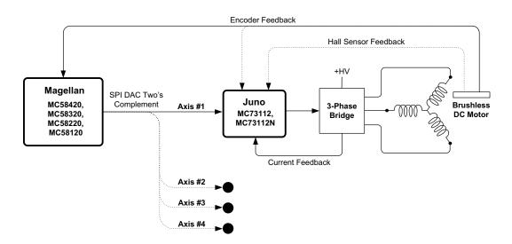
Figure 13-8: Magellan MC58000 to Brushless DC Juno Torque Control IC Typical Connections
