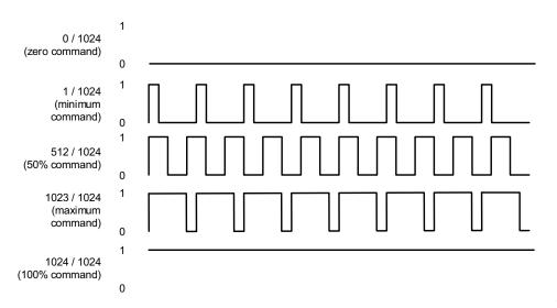
Figure 11-1: Sign/ Magnitude PWM Encoding
