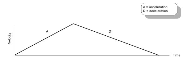
Figure 4-3: Trapezoidal Point-to-Point Profile That Doesn't Reach Maximum Velocity
