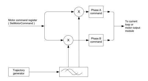
Figure 14-1: Microstepping Waveform Generation
