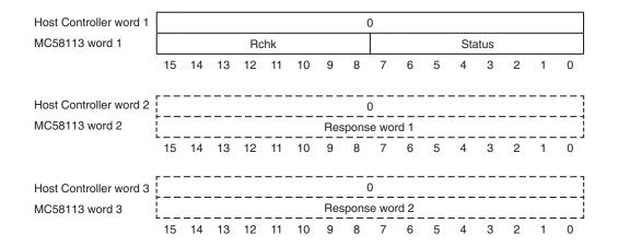
Figure 12-4 shows the packet format to receive a command response. In all cases the host sends 16-bit data words consisting of zeroes, while simultaneously retrieving data from the MC58113. The following table describes the fields of this returned data:
