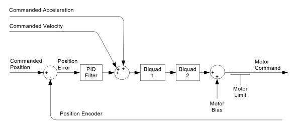
To perform position control, all servo applications require that safe and stable PID loop parameters be specified. Use of the dual biquad filters, on the other hand, is optional and will depend on the nature and complexity of the control problem. The more demanding the application, the more likely that the biquads will be useful.
