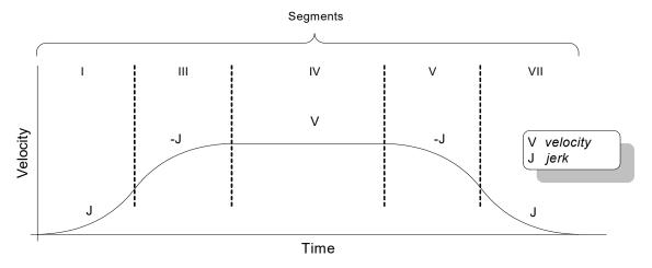
Similarly, if the position is specified such that velocity is not reached, there will be no Segment IV, as shown in <u>Figure 4-7</u>. There may also be no Segment II or Segment VI depending on where the profile is truncated.
