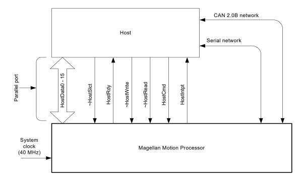
Figure 12-1: Parallel Communication Interconnection s
