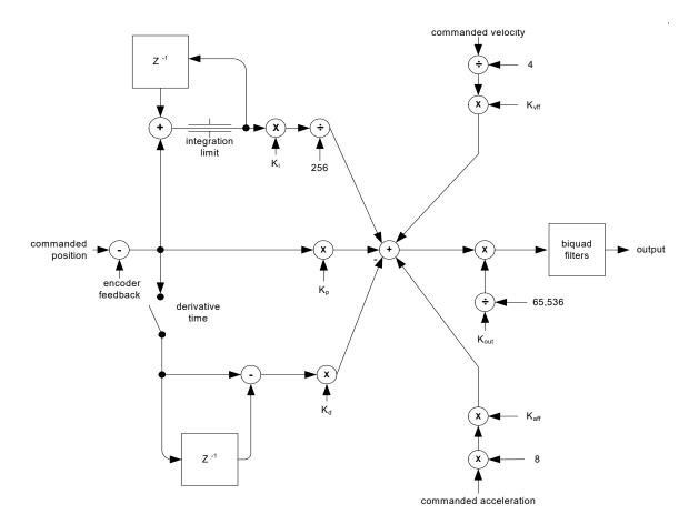
The PID+ $V_{\rm ff}$ + $A_{\rm ff}$  formula, including the scale factor and bias terms, is shown in the following equation:
