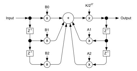
The output of the filter at time n is determined with the following equation:
