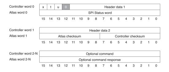
Figure 11-5: SPI Atlas Communications Protocol Overview
