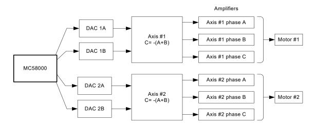
Figure 11-9: Brushless DC Motor (DAC Mode) Connection Scheme
