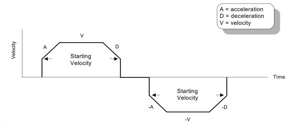
Figure 4-2: Trapezoidal Profile With Non-Zero Starting Velocity
