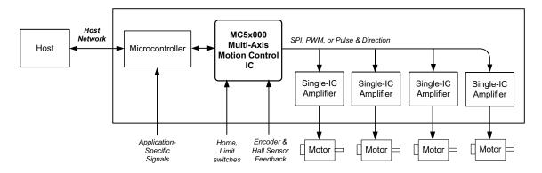
In this application the Magellan MC5x000 Motion Control IC provides high performance profile generation and position control of DC Brush, Brushless DC, and step motors. Quadrature encoders provide motor position feedback, and if Brushless DC motors are used Hall sensors provide commutation feedback. With step motors encoder feedback is optional. Additional supported signals include a home switch, directional limit switches, general purpose AxisIn and AxisOut signals, and more.
