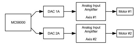
Using the DAC output mode, the digital motor output word is typically converted into a DC signal with a value ranging between –10V to +10V. This signal can then be input into an off-the-shelf DC-Servo type amplifier or into any other analog input linear or switching amplifier.
