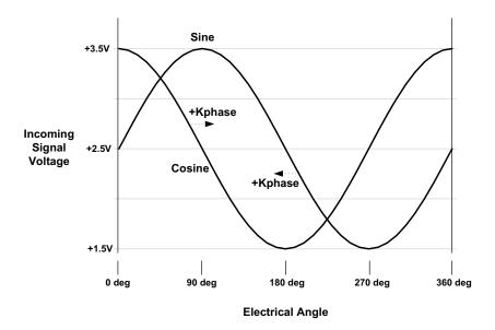
Figure 10-2: Sin/Cos Encoder Signal Waveforms
