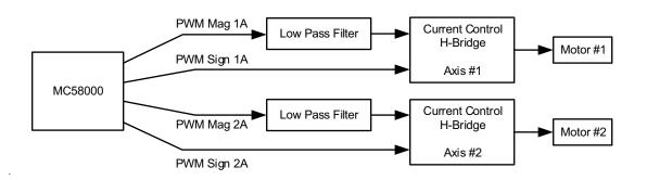
Figure 11-16: DC Brush Motor (Sign/ Magnitude PWM With Current Control) Connection Scheme
