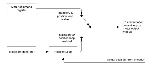
A previously disabled position loop module may be re-enabled in a number of ways. If the module was disabled using the **SetOperatingMode** command, then another **SetOperatingMode** command may be issued. If the position loop module was disabled as part of an automatic event-related action (see <u>Section 8.1, "SetEventAction Processing"</u> for more information) then the command **RestoreOperatingMode** is used.
