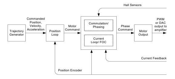
If Atlas Digital Amplifiers are utilized, then the overall control flow is modified in that the actual current loop and related drive-specific functions are located in the Atlas unit, however the Magellan IC seamlessly integrates the combined Magellan/Atlas system into one control structure which is accessed via the Magellan IC. Figure 3-2 shows the overall control flow when an Atlas amplifier is connected.
