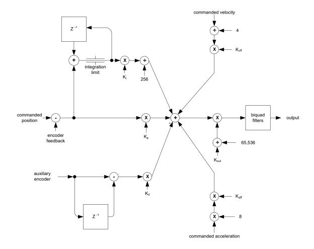
Figure 5-4: Magellan Dual-Loop Digital Filter
