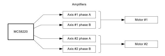
Using the DAC output mode, the digital motor output word for each phase is typically converted into a DC signal with a value ranging between –10V to +10V. This signal can then be input into an off-the-shelf DC-Servo type amplifier (one amplifier for each phase), or into any other linear or switching amplifier that performs current control and provides a bipolar, two-lead output.
