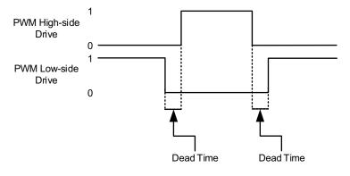
In this scheme, as <u>Figure 11-3</u> shows, the high side output and the low side output are never active at the same time. In fact there is generally a period of time when neither output is active. This period of time is called the dead time, and provides a shoot through protection function for MOSFET or IGBT switches.
