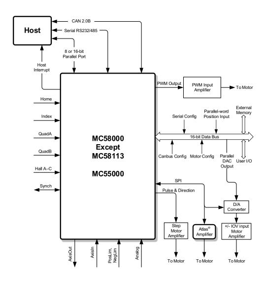
Figure 2-1: MC58000 and MC55000-Series IC Control and Data Paths
