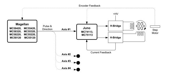
Figure 14-3: Magellan MC50000 to Juno Step Motor Control Typical IC Connections
