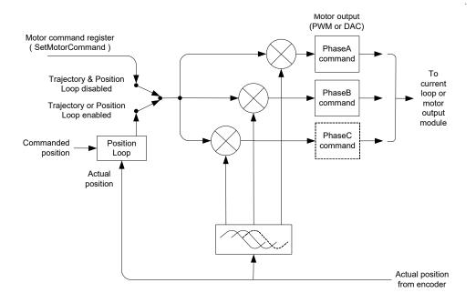
To determine the phase offset between phase A and phase B two lookup offsets are provided: one appropriate for 3-phase devices with 120-degree separation between phases (such as three-phase Brushless DC motors), and one appropriate for 2-phase devices with 90-degree separation (such as step motors). The process of determining each phase command value is called vectorization and occurs by multiplying the desired motor command by the output of the sin/cos lookup table.
