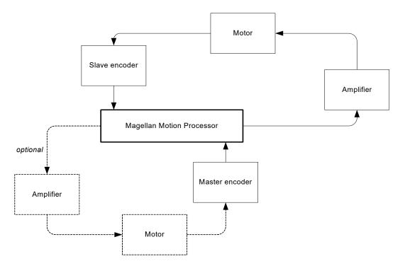
A positive gear ratio value means that during an increase in either the master axis actual or commanded position, the slave commanded position will also increase. A negative gear ratio value has the opposite effect: increasing master position will result in decreasing slave axis commanded position.
