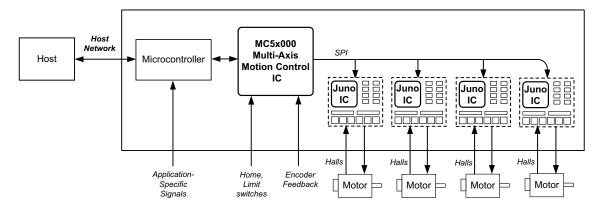
In this application the Magellan MC5x000 Motion Control IC provides high performance profile generation and position control of DC Brush, Brushless DC, and step motors. Quadrature encoders provide motor position feedback, and if Brushless DC motors are used Hall sensors provide commutation feedback. With step motors encoder feedback is optional. Additional supported signals include a home switch, directional limit switches, general purpose AxisIn and AxisOut signals, and more.
