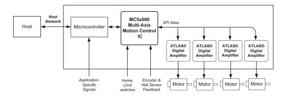
Figure 1-2: Magellan using Atlas Amplifiers with On-board Microcontroller
