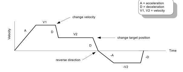
It is acceptable to change any of the profile parameters while the axis is moving in this profile mode. The profile generator will always attempt to remain within the legal bounds of motion specified by the parameters. If, during the motion, the destination position is changed in such a way that an overshoot is unavoidable, the profile generator will decelerate until stopped, then reverse direction to move to the specified position. This is illustrated in Figure 4-4.
