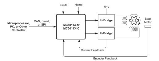
Figure 1-8: Closed Loop Stepper Operation of Two-Phase Step Motor
