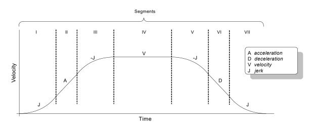
Figure 4-5: Typical S-curve Point-to-Point Profile
