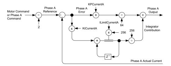
Figure 13-5: A/B Current Loop Control Flow
