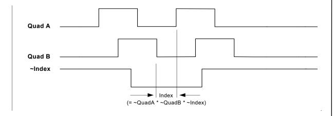
Figure 10-1: Quadrature Encoder Timing
