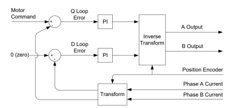
Figure 13-6: Control Flow Of FOC Control
