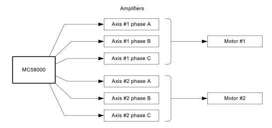
Figure 11-9 illustrates a typical amplifier configuration for a three-phase brushless motor using the DAC output mode.
