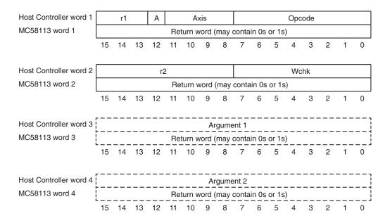
This is shown in <u>Figure 12-3</u> which shows the overall packets sequence and format for SPI command write communications. The following table details the content of these packets:
