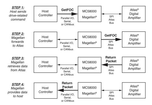
Figure 15-2: Host To Magellan To Atlas Packet Processing
