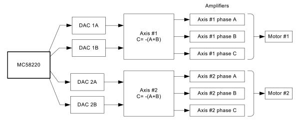
When using DAC output mode, the digital word provided by the motion control IC must first be converted into a voltage using an external DAC. Two DAC channels are required per axis. The third phase is constructed externally, using the expression C = -(A+B). This is usually accomplished with an op-amp circuit.
