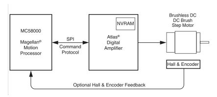
Figure 11-4: High Level Magellan To Atlas Connection Diagram
