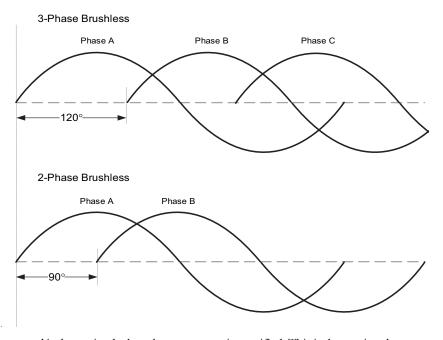
Figure 13-2: Commutation Waveforms
