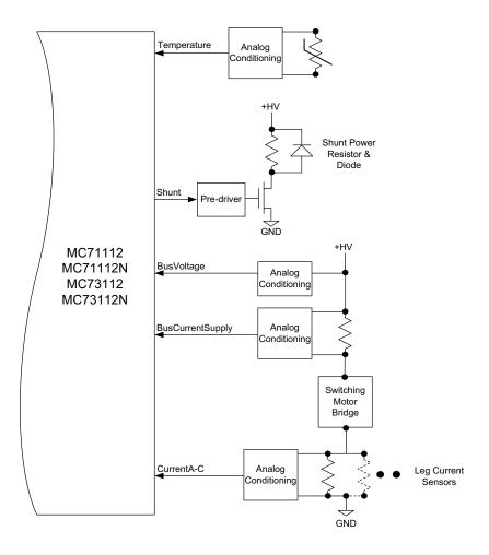
Figure 13-1: Drive & DC Bus Safety Feature Circuitry Overview
