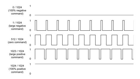
In PWM High/Low mode two output pins are used per motor or per motor phase, allowing separate high-side/low-side control of each bridge switch. In this scheme, as Figure 9-2 shows, the high side output and the low side output are never active at the same time, and there is generally a period of time when neither output is active. This period of time is called the dead time, and provides a shoot through protection function for MOSFET or IGBT switches.
