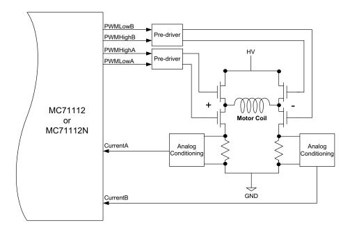
As shown in the table four PWM output signals and, if used, two analog feedback signals for current control interface between the Juno IC and the switching amplifier circuitry.
