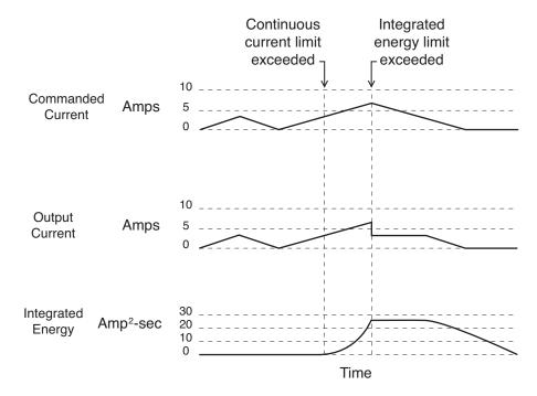
Setting continuous current limit and energy limit to less than the maximum available from the amplifier circuitry is useful if the required current limit is due to the motor, rather than to the drive electronics.
