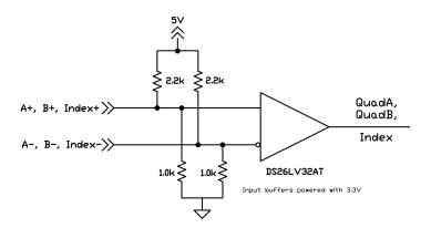
Figure 12-3 shows a typical circuit for processing differential quadrature and index signals. The pull-up and pull-down resistors provide both termination and a bias voltage. When single ended encoder signals are used connect to the positive input and leave the negative input unconnected.
