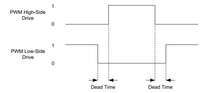
The dead time is specified in nSecs. The correct value can generally be determined from the MOSFET or IGBT IC manufacturer's data sheet, or you can call PMD technical support if you have questions.
