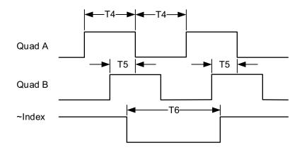
Figure 4-1: Quad Encoder Timing
