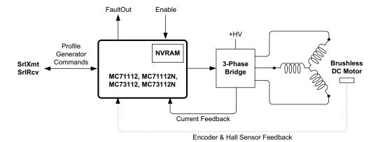
Applications: Microprocessor controlled servo motor drive, programming of Juno IC NVRAM.
