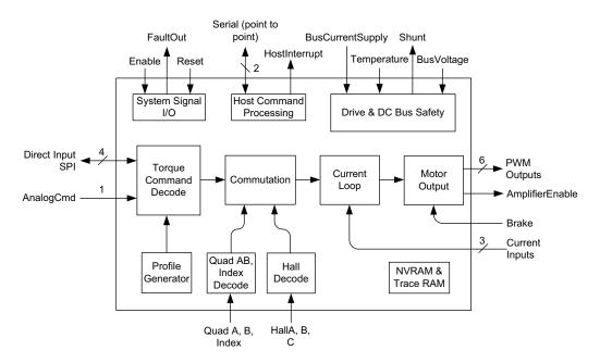
Juno torque control ICs are single-axis devices for torque or voltage-mode control of three-phase brushless DC motors and DC Brush motors.
