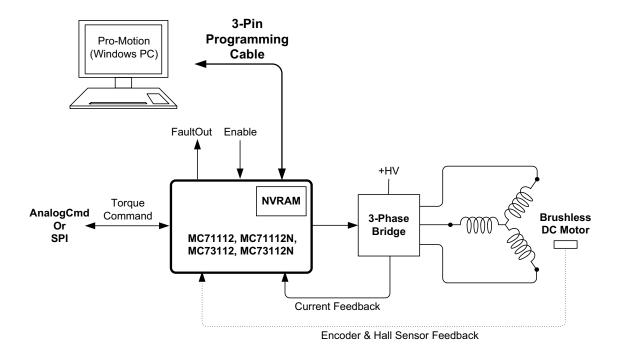
Applications: Torque Control Application Development, programming of Juno IC NVRAM
