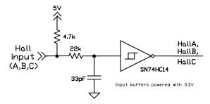
Figure 12-2 shows a typical circuit for processing Hall sensor signals. The 4.7k resistor pull-up resistor is required when the Hall signals are open-collector. The 22k resistor and 33pF capacitor provide a low-pass filter with a bandwidth of 219 kHz. The selection of the low-pass filter bandwidth depends on noise and Hall signal frequency. This buffer stage has an inversion on its output.
