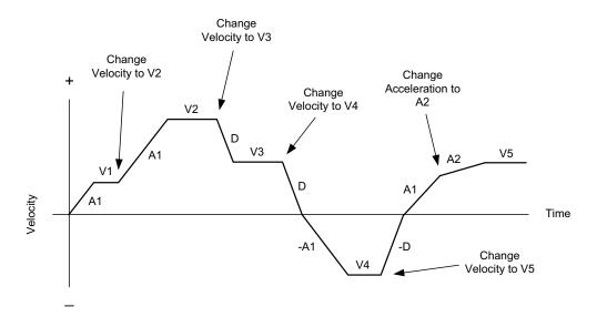
Figure 10-1: Internally Generated Velocity Profile
