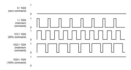
In Sign/Magnitude PWM mode two pins are used to output the motor command information. One pin carries the PWM magnitude, which ranges from 0 to 100% as shown in <u>Figure 9-5</u>. A high signal on this pin means the motor
