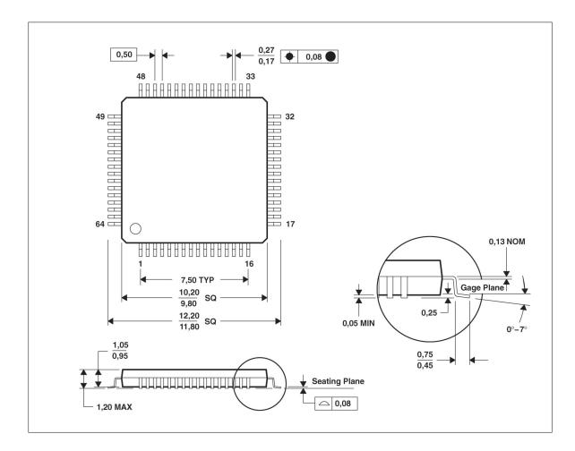
Figure 2-1: 64-Pin TQFP Physical Dimensions
