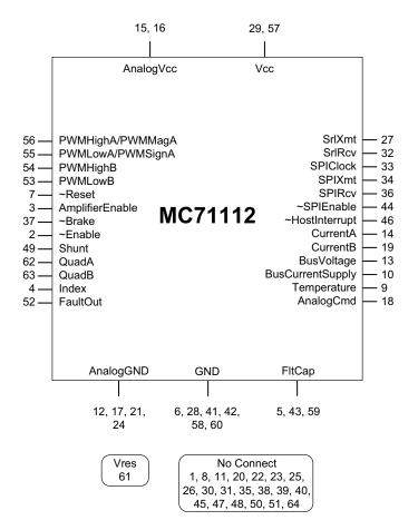
Figure 5-1: MC71112 Pinouts
