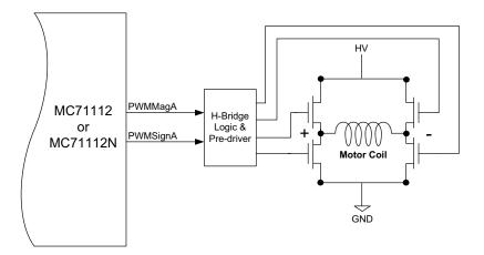
Figure 9-6 shows a typical connection for a DC Brush motor when Sign/Magnitude PWM motor output mode is used. Note that in this mode the Juno IC does not provide current control, and therefore if current control is desired this capability must be provided by the amplifier bridge's circuitry.
