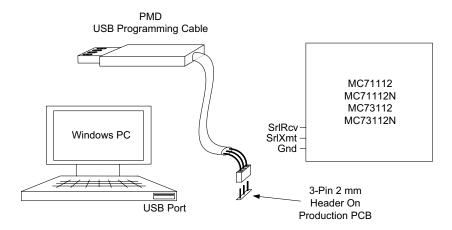
The table below shows the required wiring for the on-board connector if it is to be used with the PMD programming cable:
