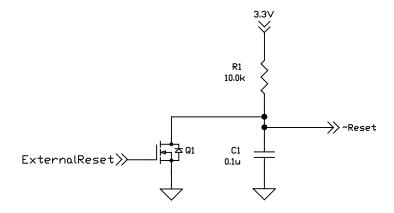
Figure 14-1 shows a typical reset circuit for the torque control Juno ICs. Although included in this circuit, external control of the Reset signal is not required since the Juno IC will trigger an internal reset upon power up. The ~Reset pin is driven low by Juno under a power-on or reset condition. If external reset is implemented an open-drain device is used. If no external reset is implemented, Q1 from the above circuit is eliminated.
