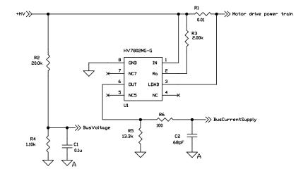
Figure 13-4: DC Bus Monitoring Circuitry
