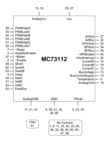
Figure 5-3: MC73112 Pinouts
