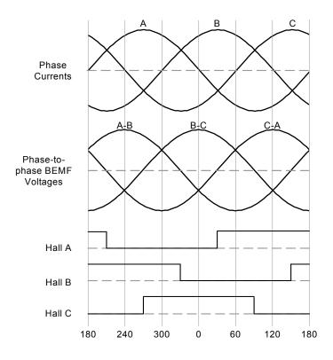
When commutating via the encoder, in addition to specifying the counts per electrical cycle Juno must determine the proper initial phase angle of the motor relative to the encoder position. This information is determined using a procedure called phase initialization. Note that a phase initialization procedure is not necessary if Hall-based commutation is selected.
