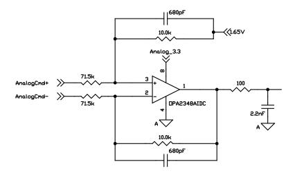
Figure 8-4 shows a typical circuit for processing a +/-10V differential input command signal. The output has an offset of 1.65V corresponding to a zero command. The bandwidth of this circuit is 23.4kHz. The 100ohm resistor and 2.2nF capacitor should be placed close to the *AnalogCmd* input pin of Juno. All resistors used should be 1% or higher grade. All capacitors should be X7R or higher grade.
