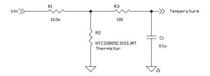
Figure 13-3: Overtemperature Processing Circuitry
