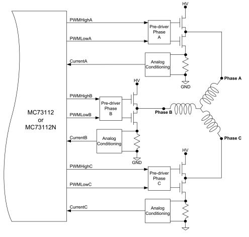
Figure 9-3: Brushless DC Motor Bridge Configuration
