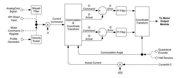
Figure 8-1: Current Loop & Commutation Control Flow
