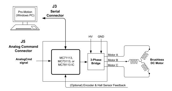
Figure 1-5: Pro-Motion Operation with External Torque Command Input
