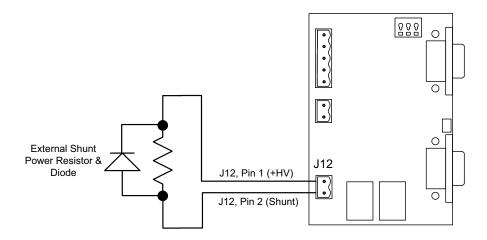
J12 provides a connection for a shunt resistor and diode that may be used to regulate overvoltage conditions on the DC bus. Such conditions can occur during deceleration of a motor with a large inertia.
