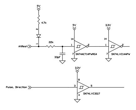
Figure 2-13: Pulse, Direction, & AtRest
