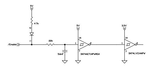
Figure 2-15: Enable Input Circuit
