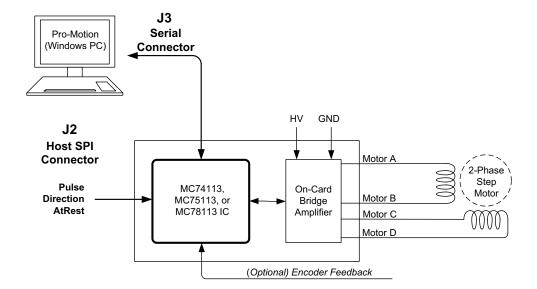
The previous first time system verification section uses the Juno Step Motor Control IC's internal profile generator to generate motion of the step motor. This is convenient because it requires a minimum of external control signals, and allows motion speeds and direction to be controlled from the Pro-Motion exercisor program.
