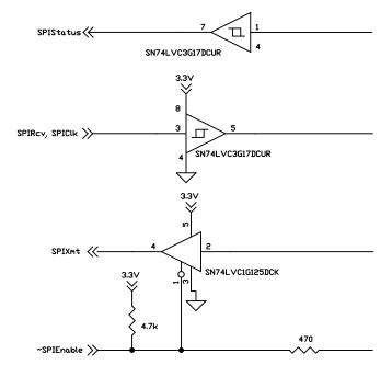
Figure 2-3: SPI Signal Circuitry
