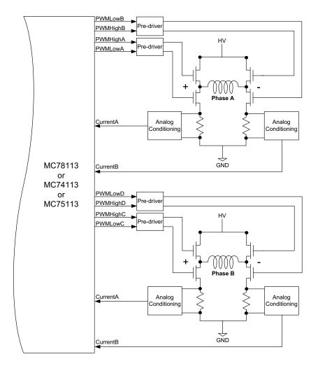
As shown in the table below eight PWM output signals and four analog feedback signals interface between the MC78113 IC and the DK78113's switching amplifier.
