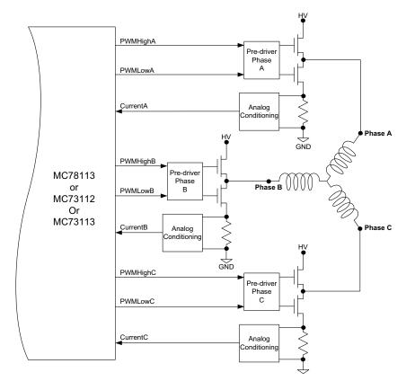
As shown in the table below six PWM output signals and three analog feedback signals interface between the Juno IC and the DK78113's switching amplifier.
