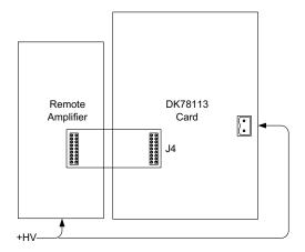
Figure 2-9: DK78113 to Remote Amplifier Board Connections
