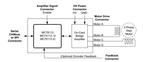
You will need to connect signals on the Axis Feedback Connector (J7), the Motor Drive Connector (J6), the Motor Power Connector (J8), and the Serial Connector (J3) to properly install the DK78113 board with an attached motor. The following three sections detail how this should be done.
