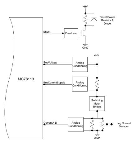
Figure 2-7 shows the DC bus monitoring circuitry used with the DK78113 board. This circuitry is designed to work with the Juno's DC bus management and protection logic. These functions include overcurrent protection, over and under voltage detection, ground fault detection, and shunt resistor control.
