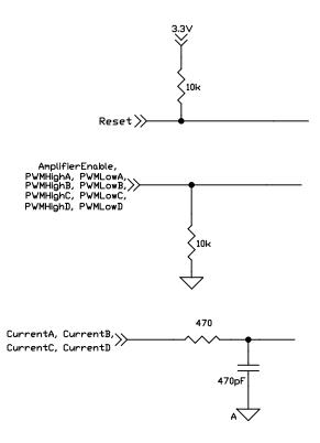
Figure 2-10: Remote Switcher Circuits
