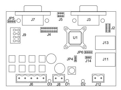
There are 14 user-accessible connectors on the DK78113 board. See <u>Figure 3-1</u> for the specific locations of the connectors on the board. The connectors and their functions are outlined in the following table:
