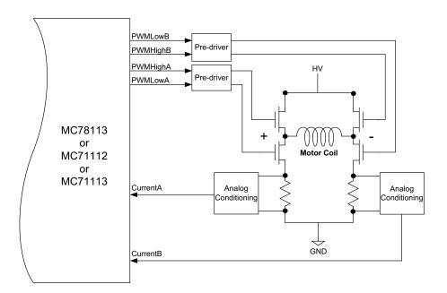
Figure 2-5: DC Brush Motor Bridge Configuration
