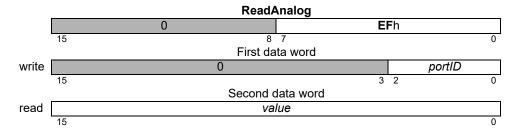
**Description** ReadAnalog returns a 16-bit value representing the voltage presented to the specified analog input. See
