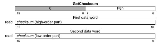
**Description** GetChecksum reads the chips internal 32-bit checksum value. The return value is dependent on the
