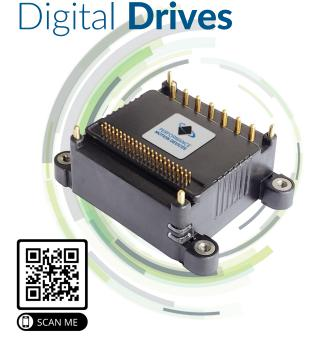
**ION/CME N-Series Digital Drives** are compact, PCB-mountable versions of PMD's ION Digital Drive family that provide high performance motion control, network connectivity and amplification. Three power output levels are available - 75, 350, and 1,000 Watts. All IONs can drive DC Brush, Brushless DC and step motors, and are ideal for medical, mobile, scientific, semiconductor, and other automation applications.
