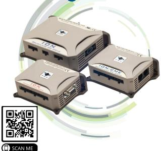
ION 500 and 3000 Digital Drives are compact, fully enclosed modules that provide high performance motion control, network connectivity and power amplification. Two power output levels are available, the ION 500 is rated at 500 Watts and the ION 3000 is rated at 3,000 Watts. All IONs can drive DC Brush, Brushless DC and step motors, and are ideal for medical, scientific, semiconductor, robotic, industrial and other automation applications.
