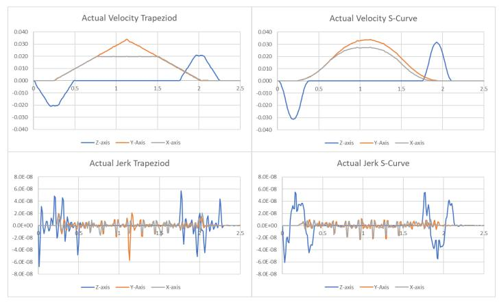
FIG 7. Figure 7. Velocity (top) and jerk (bottom) for Trapezoidal (left) and S-curve (right) profile moves.
